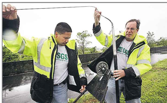
In May 2012, U.S. Geological Survey hydrologists in Bayville show how they use a probe to check for saltwater in a Lloyd aquifer well.
